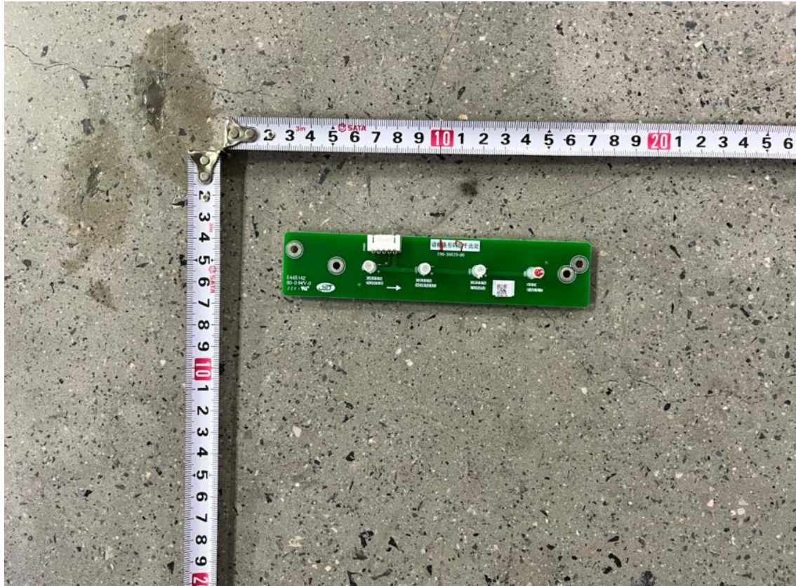
Photo 16: Front view of Lighting board:
